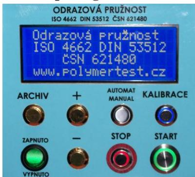
After the main switch is on the screen with basic information is displayed for 5 sec. Then the screen displays "READY FOR TESTING"
