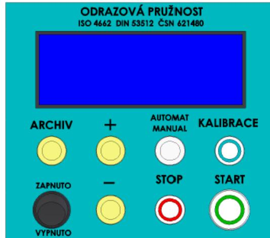
Electronic equipment consists of a pendulum angle sensor. Signals from the angle sensor are led to a display unit which calculates a value of reflection of bumper R in percentages.
