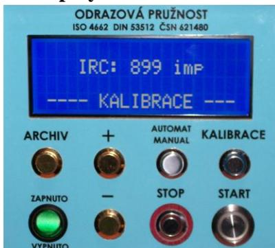
Calibration is performed only when the machine is relocated. It is sed to verify the accuracy of alignment.
