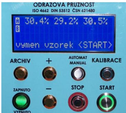
The testing for the second sample is finished
